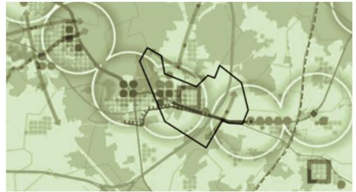
FIGURE 7. Excerpt from the SDRIF that shows priority densification areas from a regional perspective (big dots). These are mainly situated around suburban train stations (large white circles). Architects and planners working for suburban municipalities in the Paris Region use this guidance plan as a starting point for an in-depth morphological analysis of the urban fabric and of its evolution potential. Source: SDRIF (2013)
